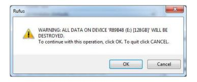
The utility will now write the ISO file to the USB flash drive. This process takes around 30 seconds to 10 minutes to complete depending on the speed of the USB flash drive.
